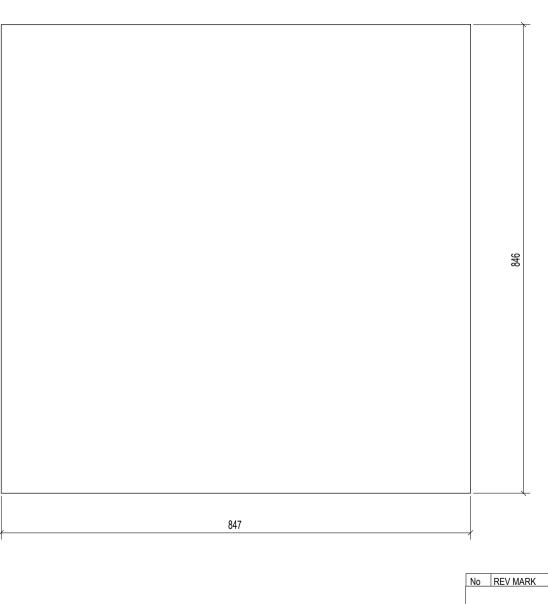
ALL HOLES ARE 22.0 mm UNLESS NOTED GENERAL NOTES: ALL WELDS ARE 6.5 mm F.W UNLESS NOTED MATERIAL LIST FOR ASSEMBLY MK'D GR/13 1 No. Required Profile No. Length Area Weight 446 PL30\*846 847 1.5 32.2 Grating Total 1.5 32.2
